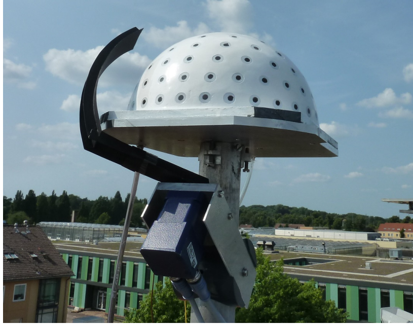
Figure 3.13: MUDIS shading unit, consisting of a stepping motor and a black shadow band.
