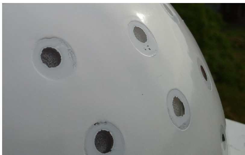
Figure 3.12: MUDIS entrance optics with condensation on the inside of the quartz glass plates.
