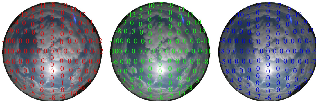
Figure 6.4: Results of an emulated MUDIS intercomparison. The three plots with the corresponding numbers, arranged like the MUDIS pattern, represent the correction factors derived for the red, green and blue channel.
