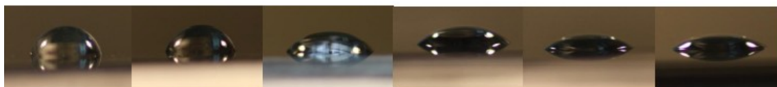
Figure 42: Photographs taken from drops of aqueous ethanol sitting on a Si wafer substrate. The concentration of ethanol ranges from 0 to 5.7 mol/l from left to right.
