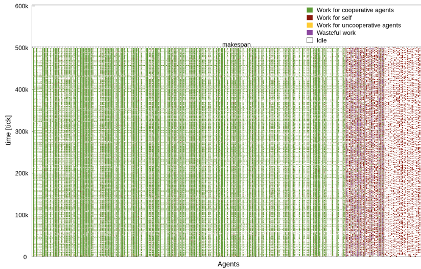
Figure 5.12: Worker diagram for the iTC -approach in the undisturbed performance experiment: The majority of agents has a high workload, working for other cooperative agents, throughout the duration of the simulation run. The second group of agents (right side) is the group of 10% EGO and FRE-agents. These agents are isolated and forced to process their own WUs.
