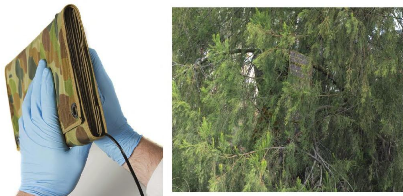
Figure 1.1 The flexible DSSC module developed by Dyesol for the Australian Army camouflages itself in trees, where it provides constant voltage under a wide range of illumination. [9]
