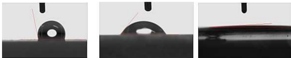
Figure 21. Different contact angle possibilities. Left: ( > 90^\circ ) poor wetting, center: ( 25^\circ ) good wetting, and right: ( < 5^\circ ) complete wetting.
