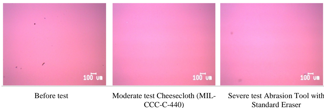
Figure 56. Nomarski-microscope magnification inspection of a 300 nm thin Suprasil substrate coated via Process V (250 °C, 2 A, 30 sccm, 0.15 nm/s). Eraser test is according to MIL-E-12397B.
