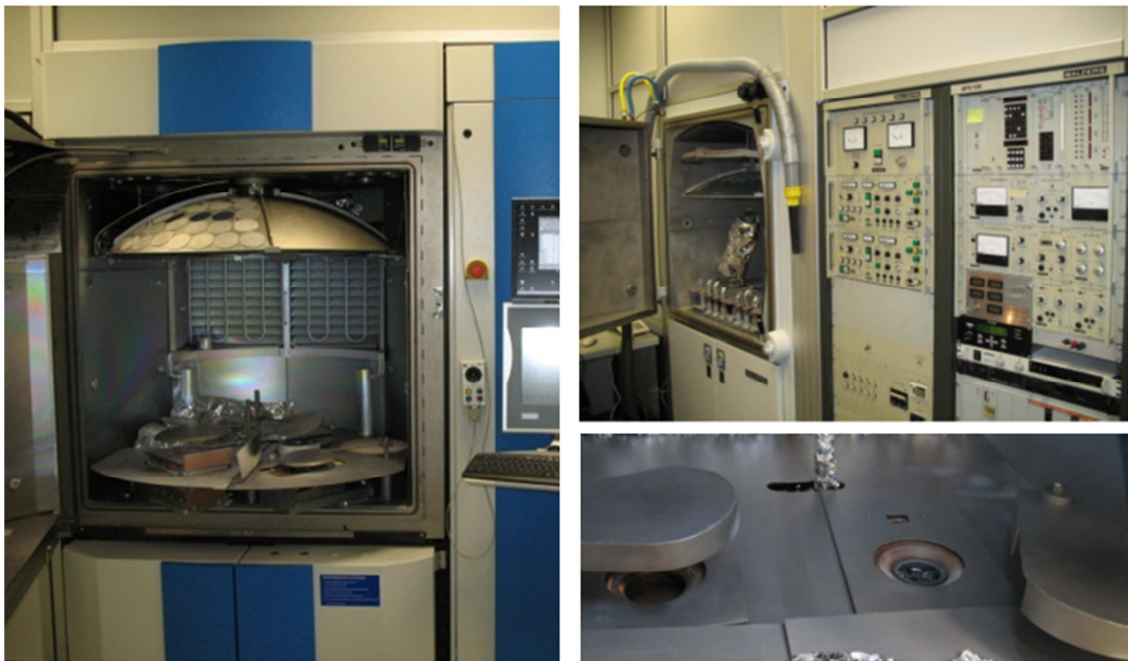
Figure 17. Thermal e-beam coating plants. Left: SYRUSpro 1100 with Advanced Plasma Source. Right: Balzers BAK 760 with Denton CC-105.
