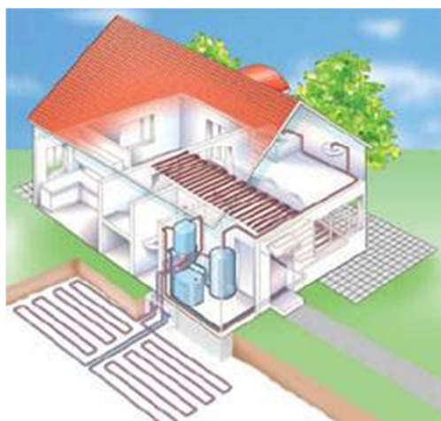
Figure 6: Geothermal horizontal loops (source: ACCLIMATIZE 2010)
