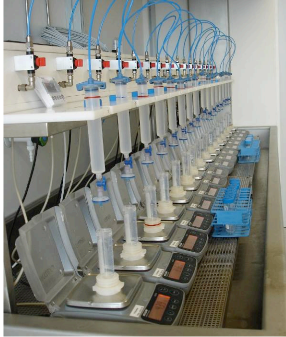
Figure 3.1: Experimental set-up used for spiking study with the bacteriophage PP7 and evaluation of the retention efficiency of virus retentive membrane material. The system allows for 16 filtration experiments in parallel.
