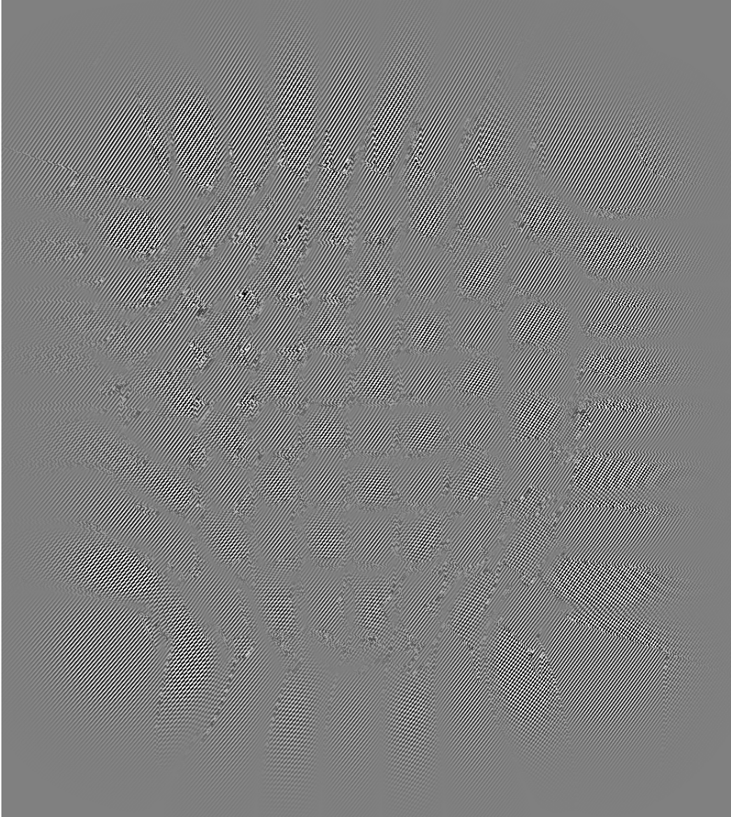
Figure 3.13: Phase hologram for \text{TEM}_{8,8} generation. This hologram is corrected by the addition of several other nominal \text{TEM}_{m,n} patterns with suitable amplitude and phase. Phase values are depicted as greyscale. The full scale (black to white) is the full actuator range of the spatial light modulator in the setup used. It corresponds to slightly less than \pi . A problem with the anti-aliasing algorithm, arising from numerical phase discontinuities, is evident in thin lines as seen e.g. in the spot in the top left corner.
