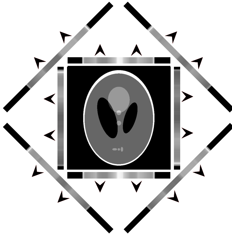
Figure 2.5 - Illustration of X-ray tomography. The central picture represents a slice of a human head with different tissues exhibiting different X-ray absorption. The slice is illuminated with X-rays from various angles. The stripes distributed around the central picture represent the X-ray shadow for the corresponding angle. From these shadow images the central image can be reconstructed via the so called inverse Radon transform.
