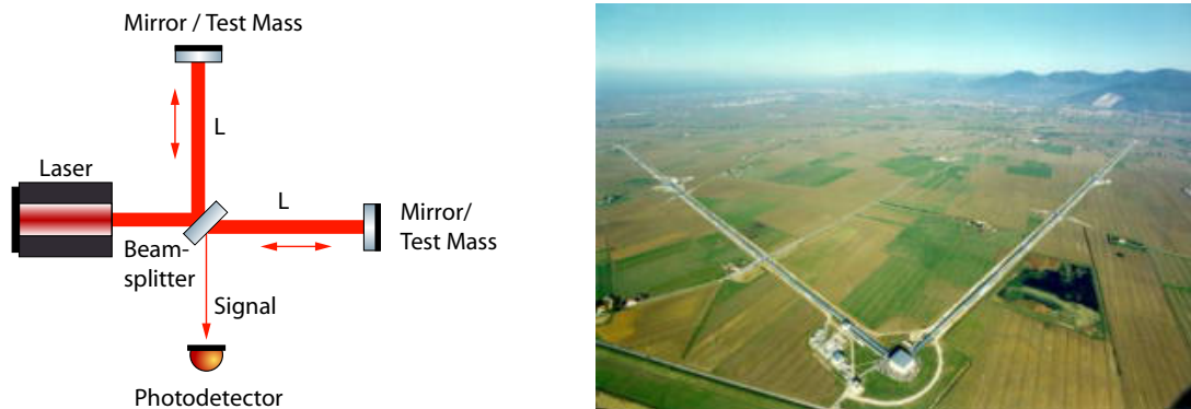
Figure 1.1 — Left: A classic Michelson interferometer consists of a laser, a 50/50 beamsplitter, two test mass mirrors and a photodetector. One can think of the gravitational wave as modulating the effective refraction index of the vacuum, thereby shortening the length of one arm while expanding the length of the other. Right: Photograph of the French-Italian VIRGO detector with an armlength of 3 km.
