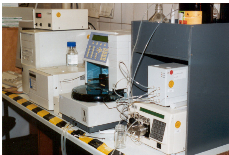
Figure 3.2 Instrument of amino acid analysis, HPLC; RF 10AXL fluorescence detector, Shimadzu; Resolve TM 5 \mu m C 18 , 4 \times 150 mm, Reversed phase Waters.
