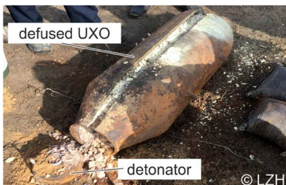
Fig. 1 UXO defused by low order detonation
