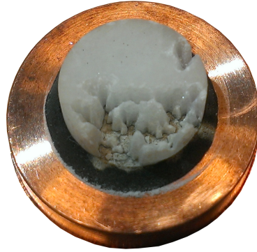
Figure 7.8.: ^{39}\text{K}^{37}\text{Cl} ablation target after several 1000 ablation shots showing the disrupted surface structure. The target is mounted with cryogenic glue (black) on the targetholder made of oxygen free copper.
