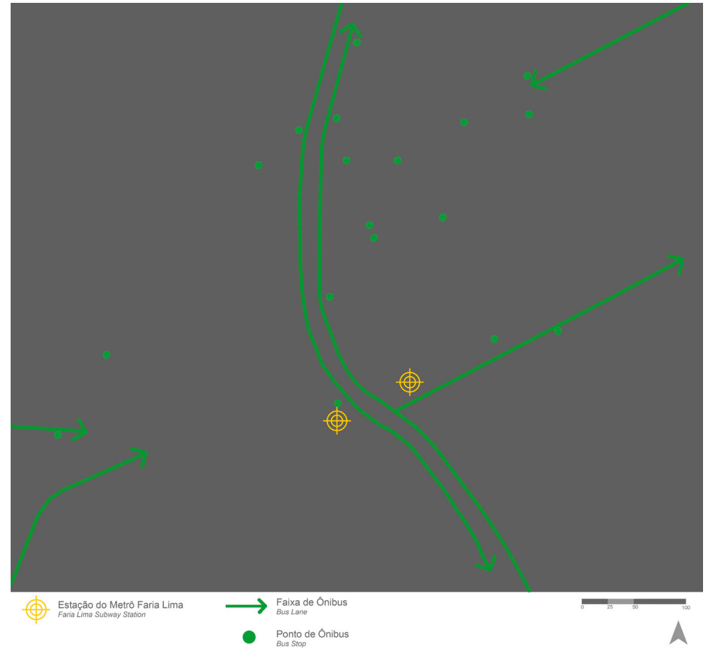
Figure 65 Diagram of the microaccessibility by bus to the Faria Lima station. Source: author, 2017.
