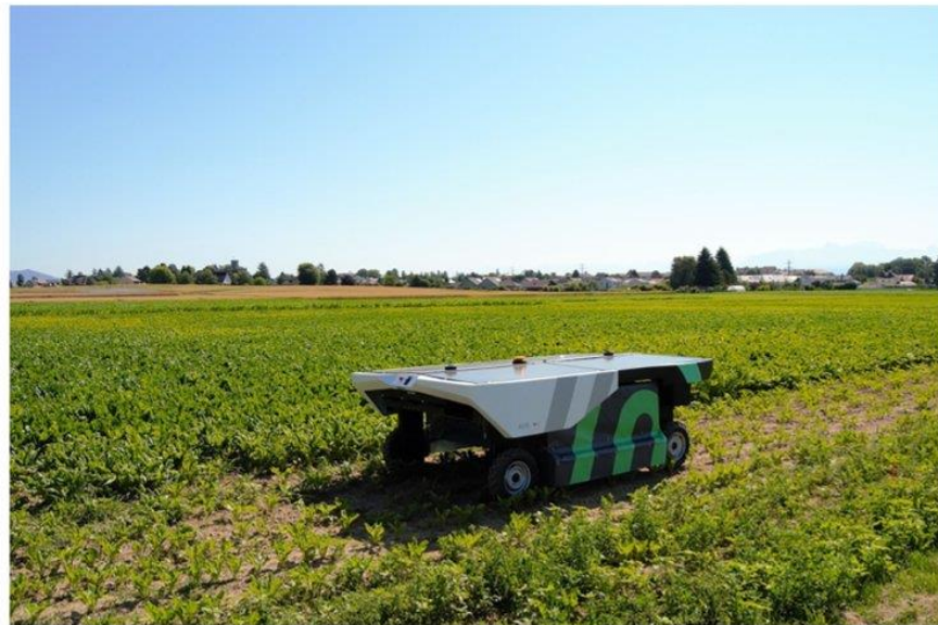
Fig. 1 Autonomous weeding machine (AVO) from ecoRobotix. Photo available for download from https://ecorobotix.com/en/contact
