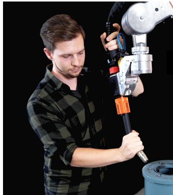
Figure 7.1: Example for human-robot interaction with a collaborative robot. Image source: voraus robotik
