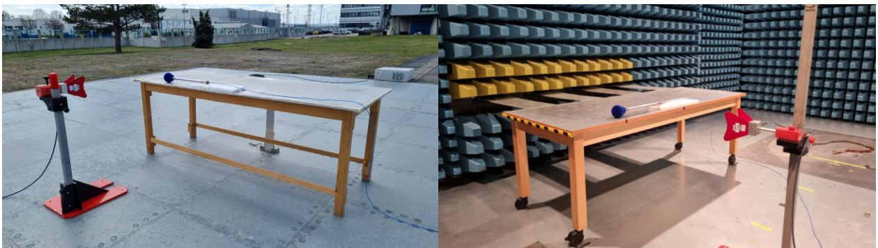
Figure 5: Validation setup on OATS and inside ALSE, horizontal antenna polarization
