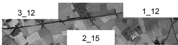
Figure 1: Overlay of corresponding SkySat Basic images captured by the SkySat SSC12's three CMOS-frame sensors
