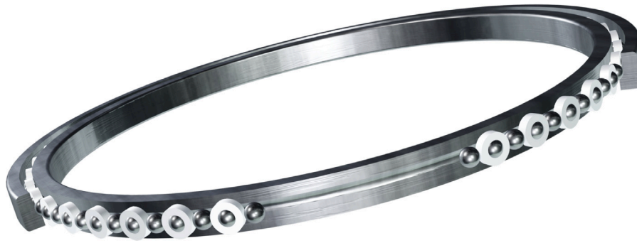
Fig. 17. Thin cross-section angular contact bearing with polytetrafluorethylene (PTFE) toroidal ball separators, commonly used in space applications as pre-loaded pairs.
