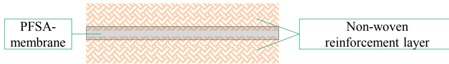
Figure 2: Schematic representation of the sandwich membrane
