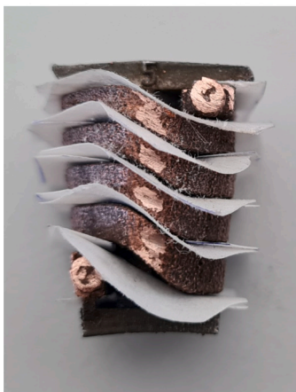
Fig. 13. Coil after the thermal treatment and adding isolation paper between the coil layers.
