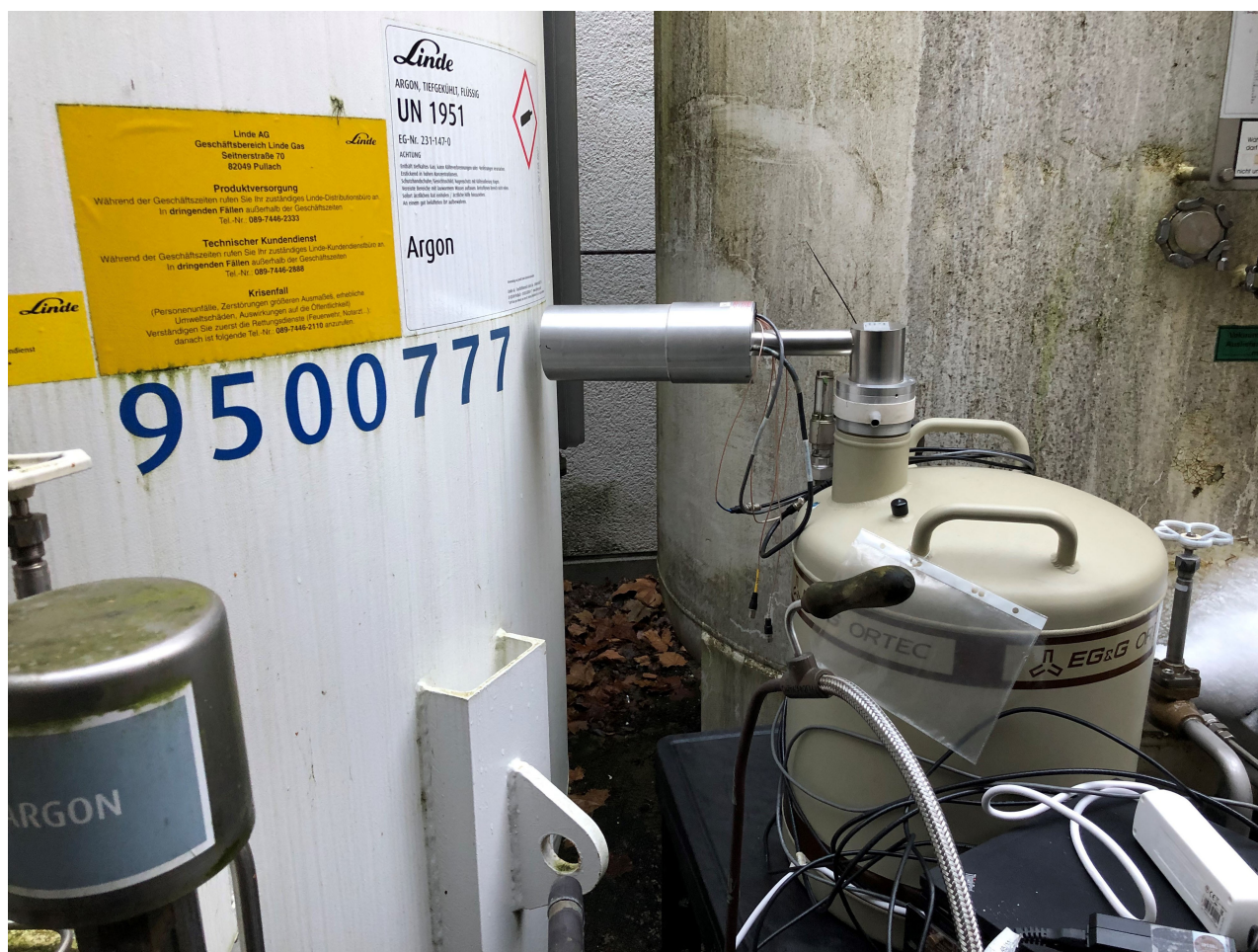
Figure 5. Measurement setting of gamma emission from the argon tank.
