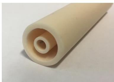
**Figure 2.** Radiation protection of the thermocouple
