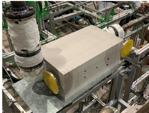
**Figure 4.** Close up of the insulated additively manufactured plate-fin heat exchanger
