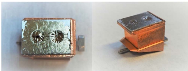
Figure 3. Photographs of an aluminum support covered with a 50 nm thick self-supporting carbon foil mounted on a wedge-shaped DESY copper sample holder. In the top view on the left, the dark spot in the center of the left aperture is an AuNP sample deposited by the drop-casting method. The part of the carbon foil covering the right aperture was used for reference measurements.
