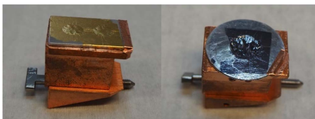
Figure 4. Photographs of the other samples used in the measurements mounted on wedge-shaped copper DESY sample holders. Left: A 100 nm thick gold foil attached to an aluminum support with two 5 mm apertures. Right: The 5.3 nm AuNP sample provided by Université de Namur.
