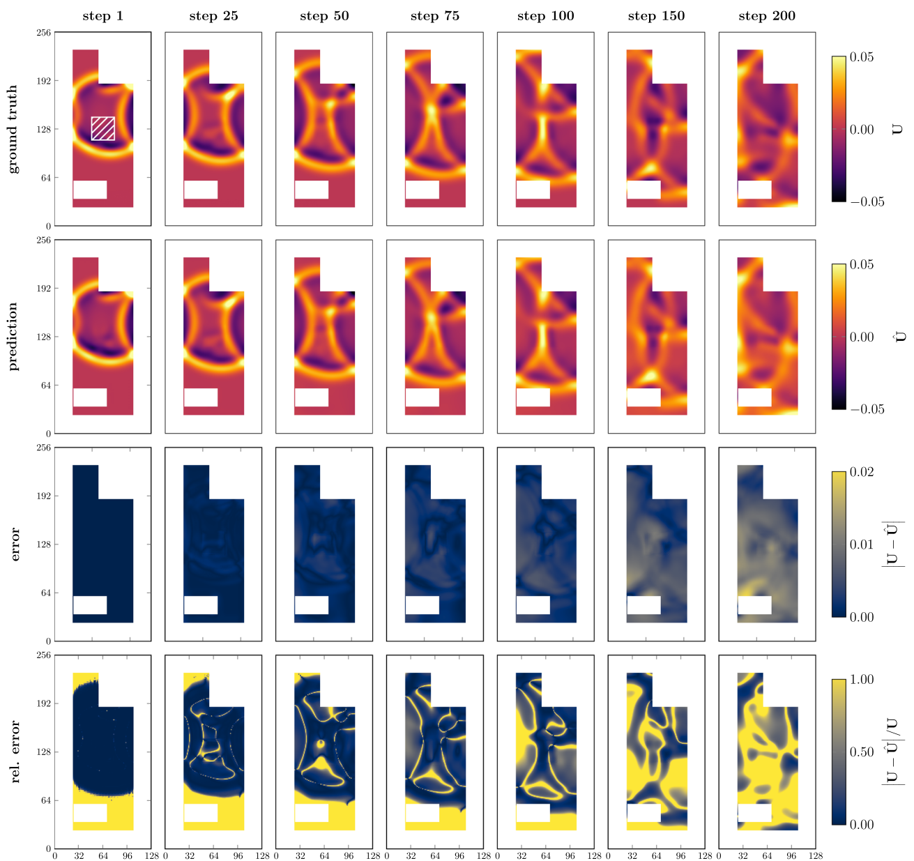
Fig. 5 Evolutions and predictions of wave dynamics in a complex and heterogeneous domain using the \mathcal{U}_{64}^3 model. The material inhomogeneity is indicated by the hatched patch in upper left panel. The first prediction is initialized from wave fields at time steps t = 1.47, 1.48, 1.49 s from validation case (f). From there on, recursive time
