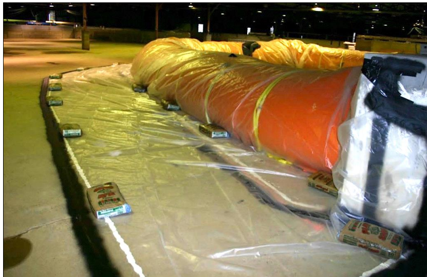
Abb. D-15: Tiger Dam – Testaufbau vom Tiger Dam (42") im Engineer Research am Development Centre vom US Army Corps of Engineers in Vicksburg (Ward, 2013)
