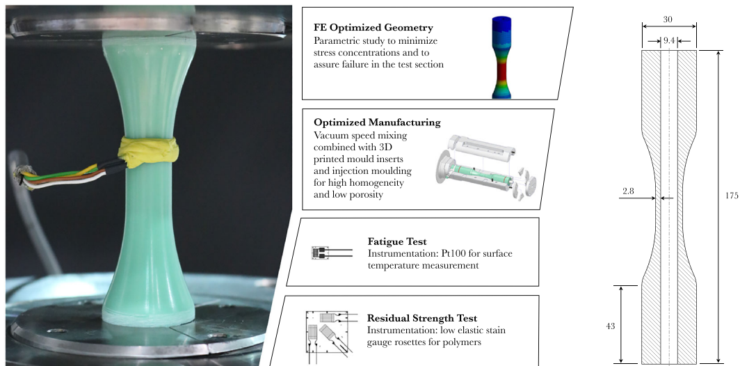
FIGURE 1 Test setup for every fatigue test conducted. A Pt100 sensor is used to measure the surface temperature. In case a run-out is declared, a residual strength test is performed using strain gauge rosettes. 16 Optimization processes related to the specimen geometry and manufacturing were presented in a previous publication. 12 Dimensions in mm. [Colour figure can be viewed at wileyonlinelibrary.com ]
