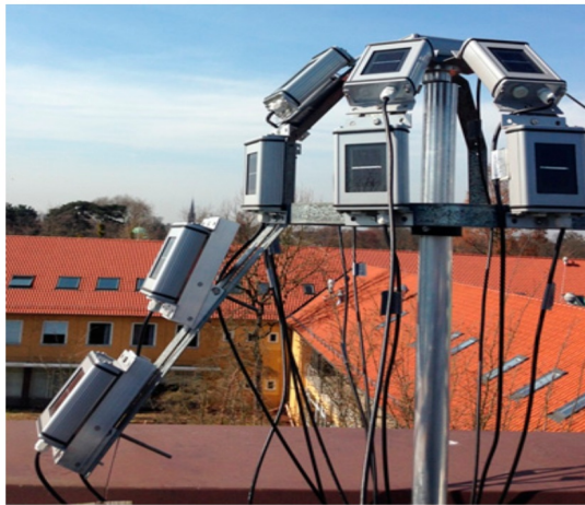
Figure 6.4: Radiation sensors on the roof of the IMUK building. Image taken from [63].
