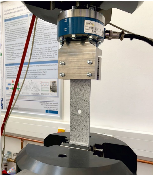
Fig. 12 Test sample clamped into test machine
