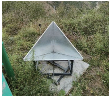
Figure 5.7: Site photos of the interference TCR near our tested CR03.
