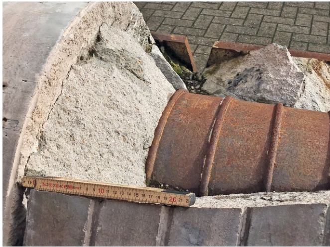
Fig. 6 Opened test body of a grout connection
