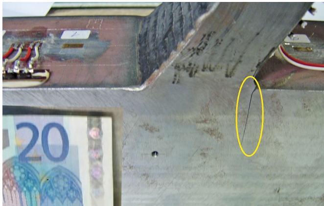
Fig. 8 Test body of a fatigue-stressed weld with cracking clearly visible
