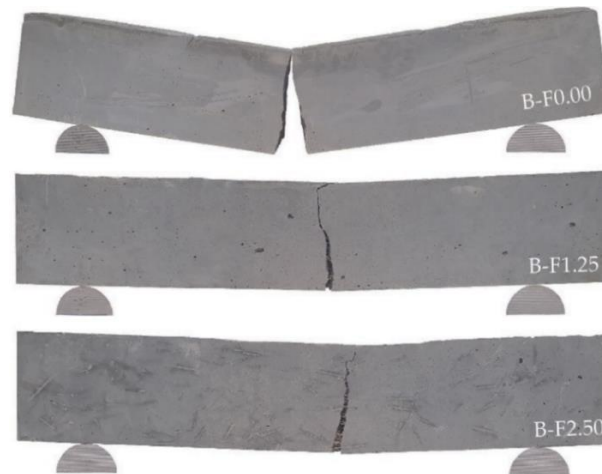
Figure 6. Crack patterns after the test (side view).
