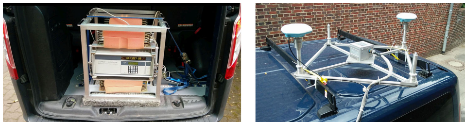
FIGURE 5 Parts of the measurement equipment: on the left, passive hydrogen maser (PHM) placed inside the trunk; and on the right, an inertial measurement unit (IMU) and GNSS antennas mounted on the roof of the vehicle [Color figure can be viewed in the online issue, which is available at wileyonlinelibrary.com and www.ion.org ]
