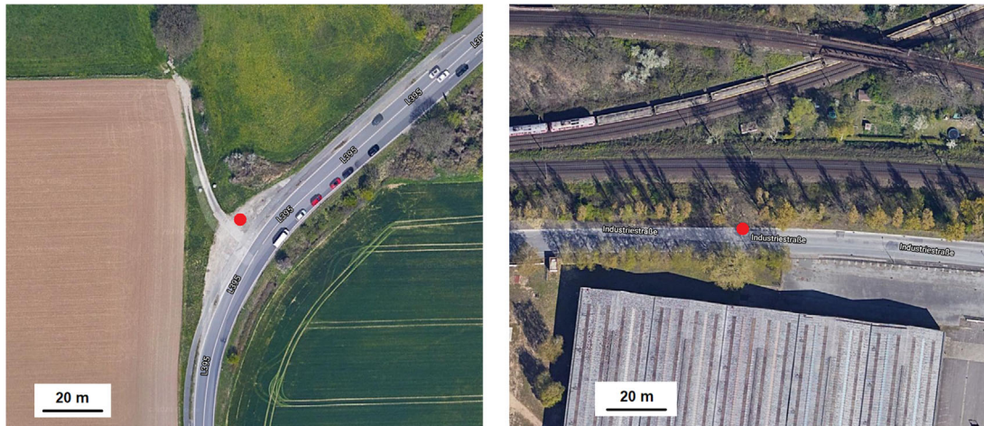
FIGURE 7 Locations where static data were recorded indicated by red dots: good observation conditions on the left, and suboptimal conditions (row of trees to the North, building to the South) on the right (map source: Google Maps) [Color figure can be viewed in the online issue, which is available at wileyonlinelibrary.com and www.ion.org ]
