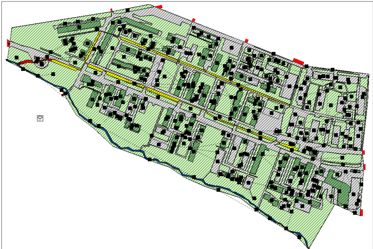
EPA SWMM model set-up for the study area Vauban. The colours represent land uses. Light green: Green Areas, Dark green: Green roofs, Grey: Sealed Areas, Yellow: Swales, Red: Outlets, Blue: Waterbodies. Master Thesis by Karina Sináí Medina Camarena.
