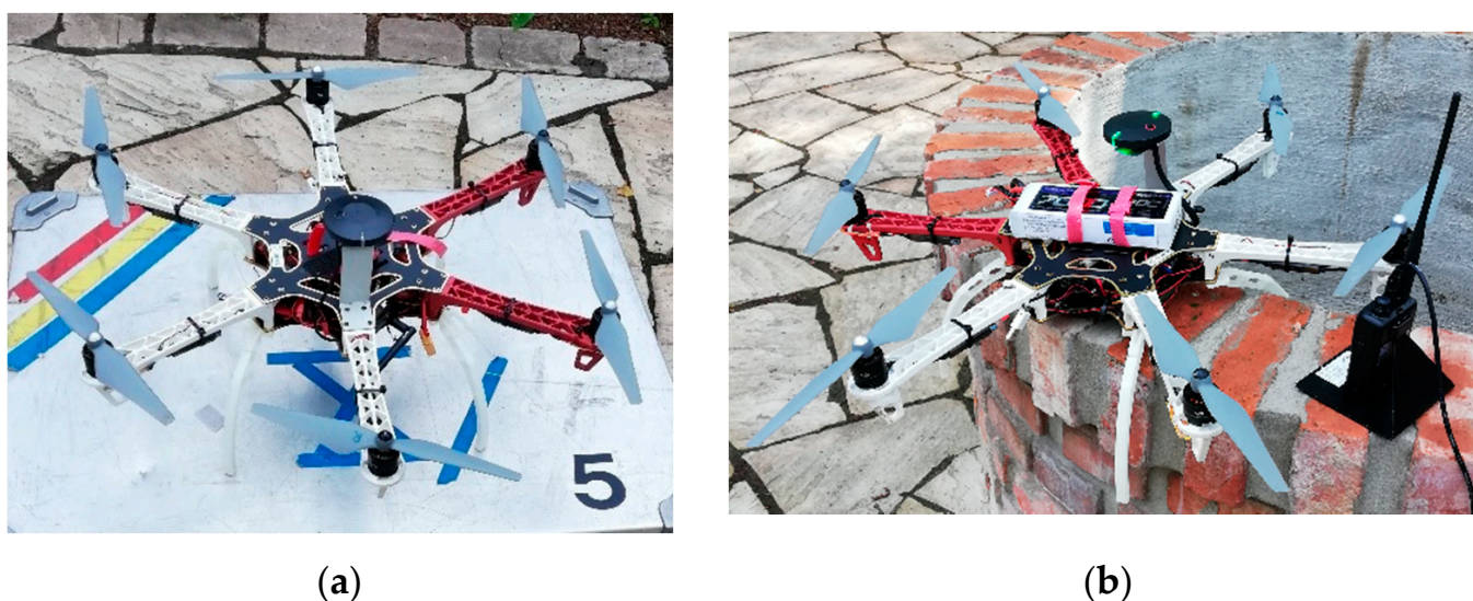
Figure 3. Drones from IMuK for measurements in the green and blue courtyard (a) for vertical probing and (b) for infrared measurements.
