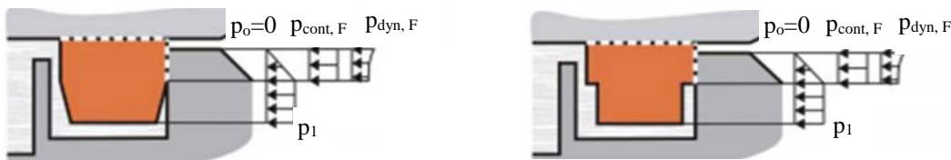
Figure 2.15: Hydrostatic load reduction via chamfers (left) and pockets (right) [83].
