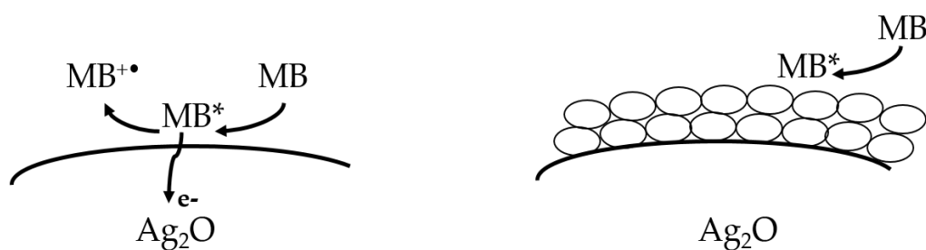
Figure 5-10. Proposed mechanism for MB bleaching over Ag 2 O, Ag 2 O-containing mixtures, and composites under vis-light illumination. This figure is a reprint of Figure 2-7 in Chapter 2 (page 54).
