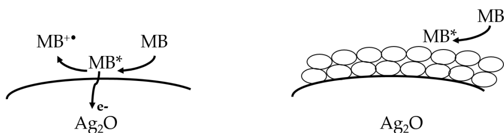
Figure 2-7. Possible mechanism of MB bleaching by Ag 2 O and Ag 2 O-containing mixtures and composites under visible light illumination.
