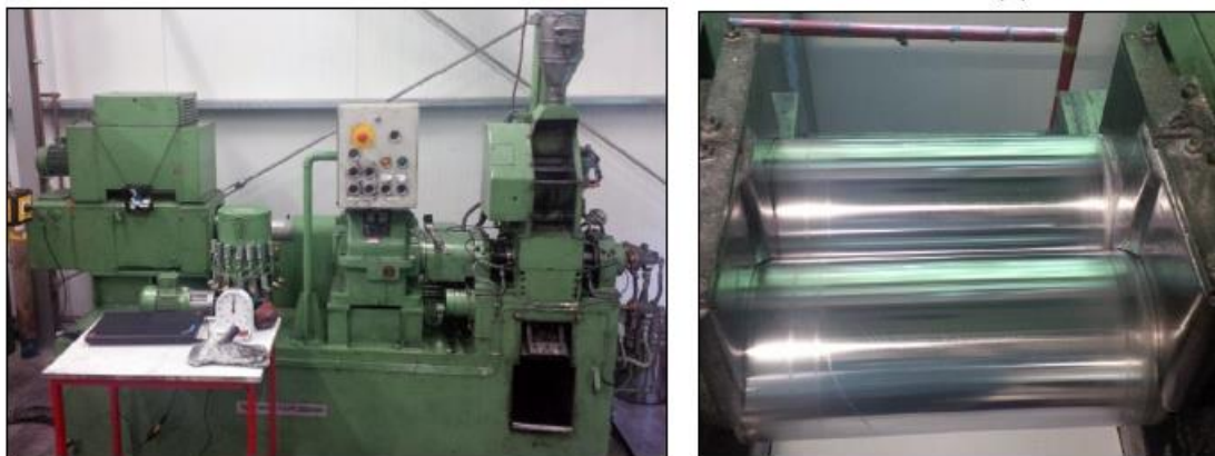
Figure 70. Representation of the internal mixer (left) and the rolling mill (right) for the production of the mixtures.
