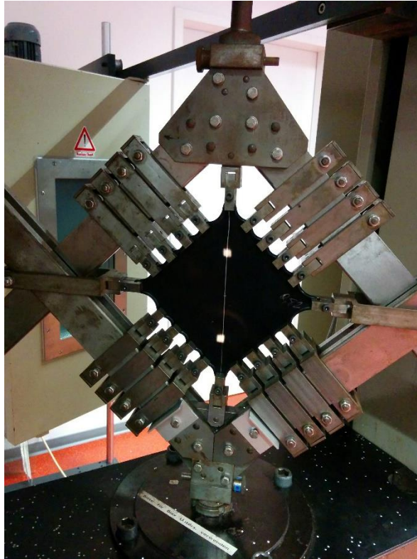
Figure 76. Equi-biaxial test performed in the Zwick machine.
