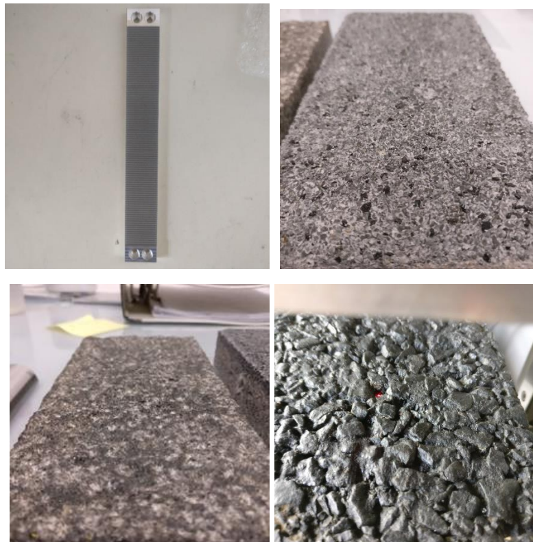
Figure 82. Types of substrates used for the friction investigation.
