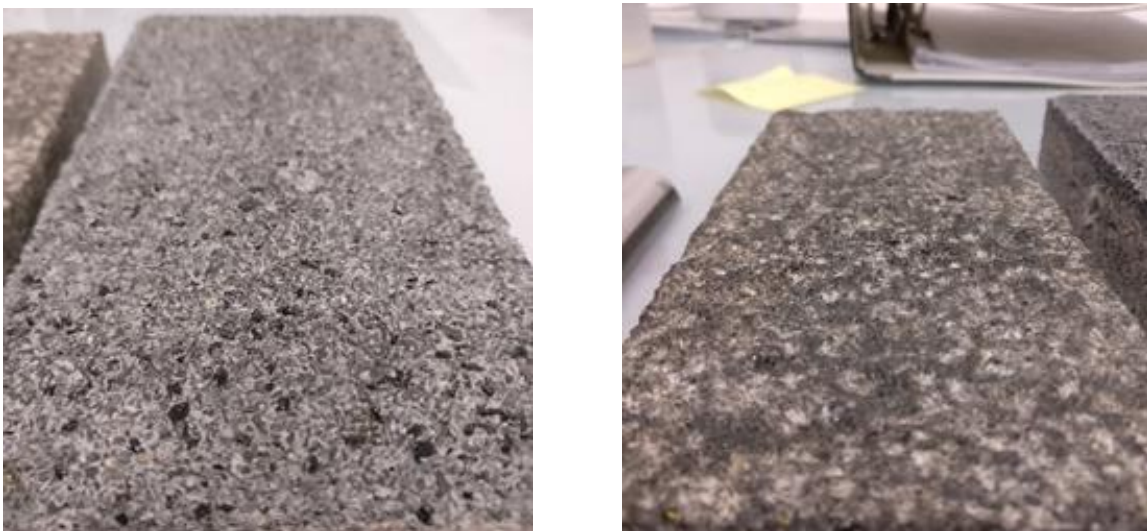
Figure 97. Rough substrates used for the investigation: fine granite paver (left side), rough granite paver (right side).
