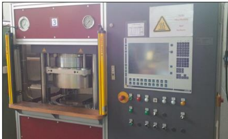
Figure 73. Heating press used for the vulcanization process of the compounds.
