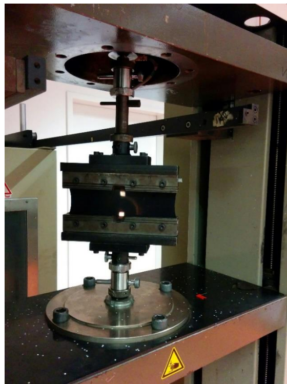
Figure 75. Multihysteresis test in shear mode.
