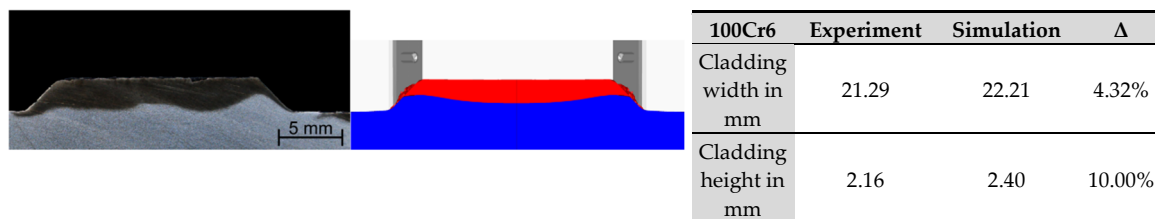
Figure 28. Comparison experiment/simulation 100Cr6, 27 mm base cylinder, 15 mm cladding width.
