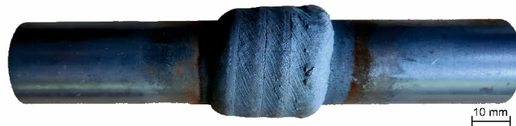
Figure 7. Welding seam after cladding by PTA.
