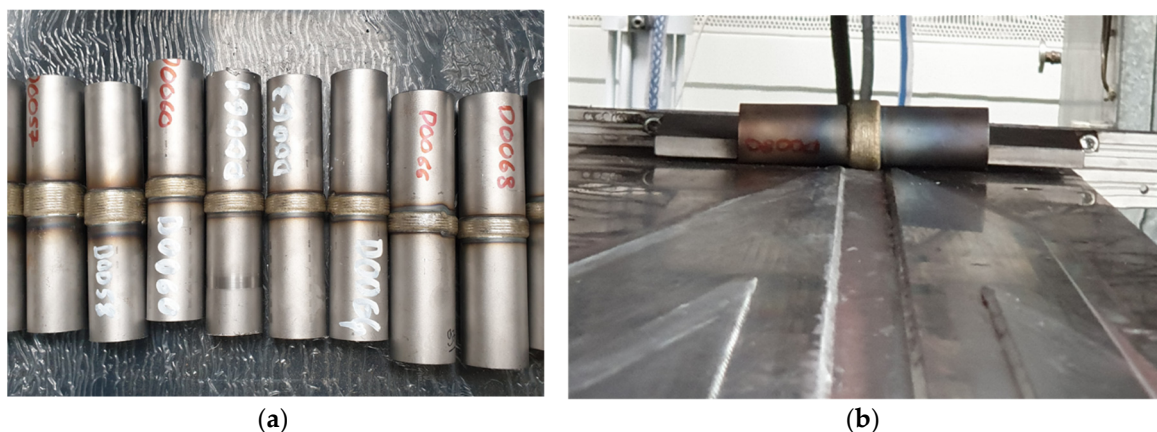
Figure 18. (a) Work pieces with different amounts of cladding; (b) (cold) work piece in starting position.
