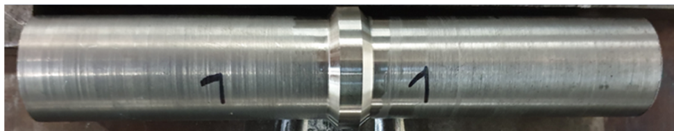
Figure 14. Work piece 100Cr6/C22.8 milled to 27 mm diameter and 10 mm cladding material seam.
