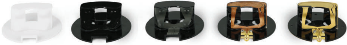
Figure 2.4 Plastic part in different LDS processing steps - SLA part (only for LPKF ProtoPaint), injection moulded or ProtoPaint SLA part, laser structured part, metallized with LDS copper and metallised with surface finish (NiP/Au)
